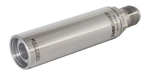
The Imenco Greytip Shark Subsea Camera is small size camera delivering high quality SD video, used where space is a restricting factor. The Greytip is preferred by dive companies and ROV operators as a tool / inspection camera. A high resolution color camera module is built into the small duplex steel housing, enabling the Greytip Shark to withstand pressures down to 6,000MSW.
