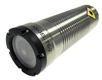
The Imenco Angel Shark T6-2 150mW Subsea Green Line Laser is the most powerful underwater survey laser available in the market. Primarily used for survey of underwater pipeline & underwater structure inspections. By mounting two lasers in a fixed bracket, calibrated at a set distance, measurements can be picked out from subsea video.
