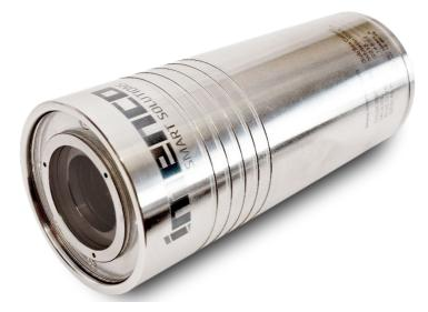
The Imenco Blacktip Shark<sub>HD</sub> Colour Zoom Camera incorporates a 4Mpx - 1/3" CMOS sensor and features a 10x optical zoom lens. With its ultracompact and lightweight Titanium body rated to 4.000msw, it is an ideal camera for inspection of restricted spaces and for use in tooling applications.
