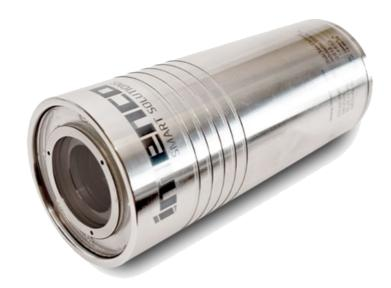
The Imenco Blacktip Shark II Colour Zoom Camera incorporates a 1/3-type CMOS and features a 10x optical zoom lens (+ 16x digital zoom). With its ultra-compact and lightweight Titanium body, rated to 4.000msw, it is an ideal camera for inspection of restricted spaces and in subsea tooling applications.
