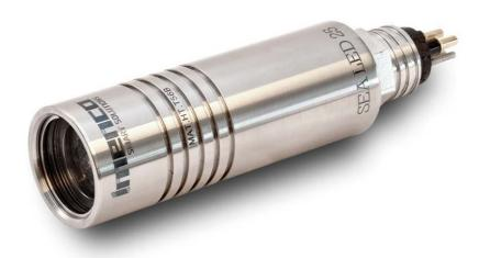
The Imenco SeaLED 25 is a high output multipurpose Subsea Light for ROVs, tools, inspection points and divers. Fitted with the latest high quality LED which produce an increased lifespan compared to the traditional Halogen and HID lights. The SeaLED 25 can be delivered with different colour temperatures and lens angles. The light output is easily regulated from 0-100%.
