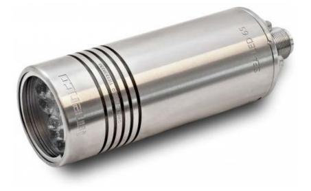
The Imenco SeaLED 65 is a high output multipurpose light for ROV / tools and inspection points. Equipped with the latest high quality LED and built in temperature protection which produces an increased lifespan compared to the traditional Halogen and HID lights. The light output is easy regulated from 0-100% by different regulation methods, including remote control option.
